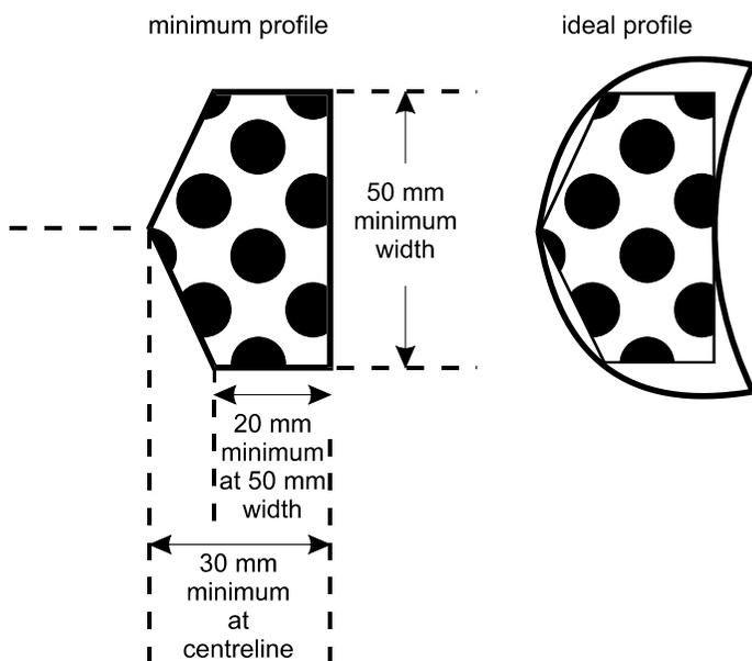
1.4. The padding must be positioned on the edge (see definition of edge in kayak specifications) to cover at least 15 mm above and below the edge.
